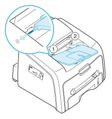
Fold out the extender, if necessary.
